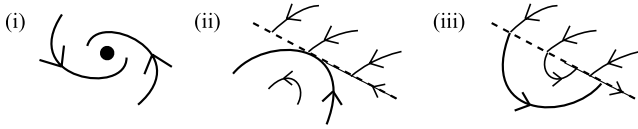
Fig. 1. Simple singularities: (i) a stationary point, (ii)–(iii) tangencies between a flow and a line of discontinuity (dashed), known as (ii) a visible fold or (iii) an invisible fold.
